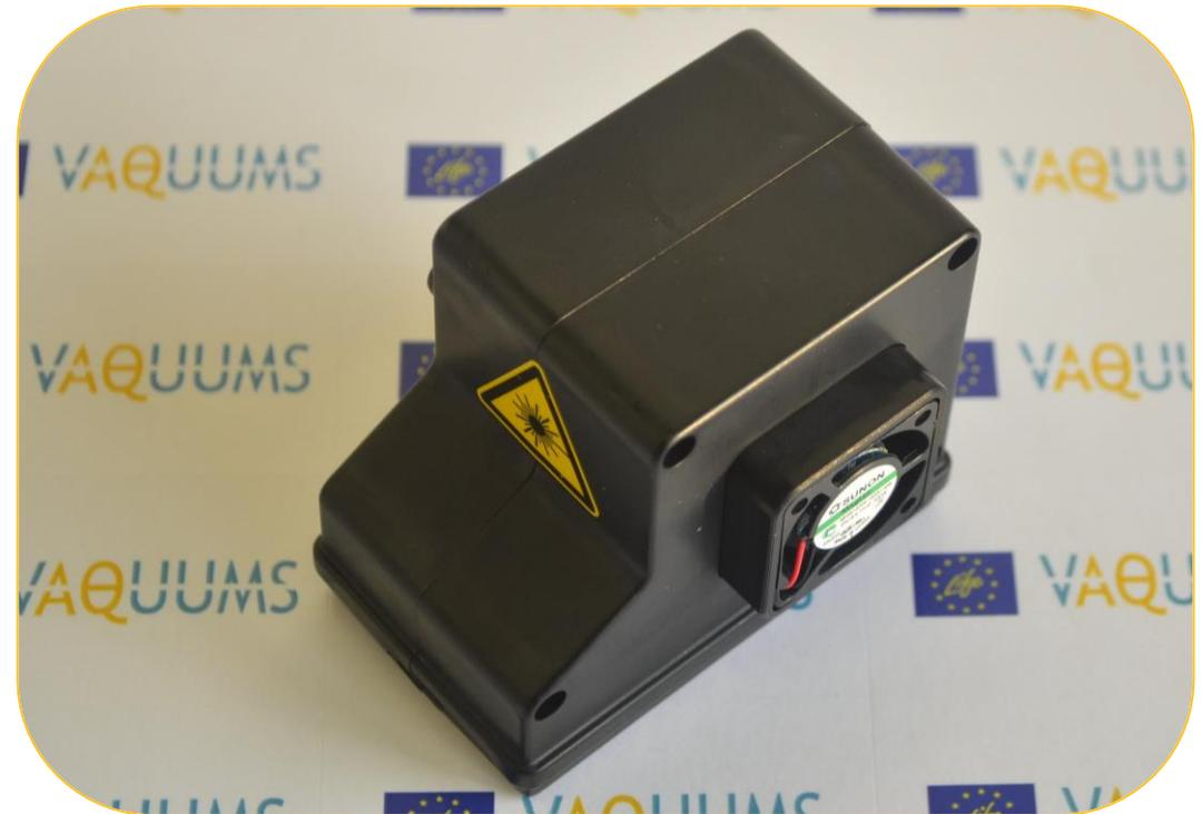
The Alphasense OPC-N2 is an optical particle counter. According to the manufacturer, the flow correction of this sensor ensures stable readings, even in high dust environments. The OPC-N2 measures particles from 0.38 micron to 17 micron diameter at a 1 second interval. The OPC-N2 provides both PM readings and real time particle size histograms.
