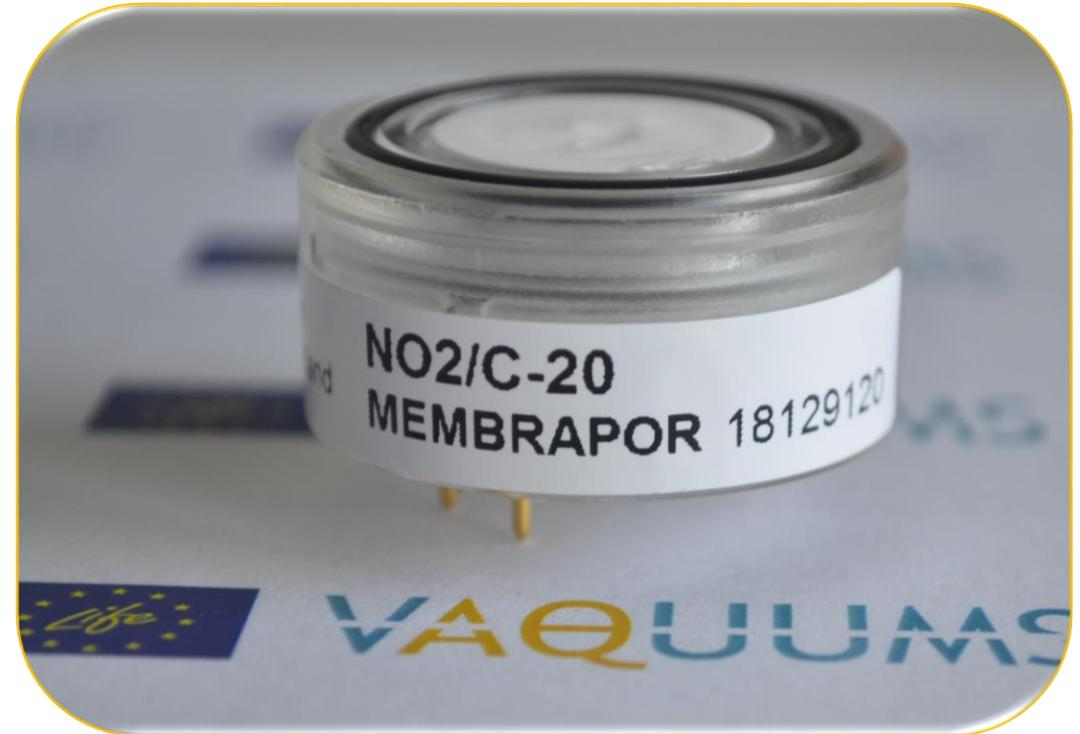
The Membrapor NO<sub>2</sub>/C-20 is an electrochemical nitrogen dioxide sensor. It can measure concentrations between 0 and 20 ppm. According to the manufacturer the compact series have the highest reliability and maximum performance in a compact housing. The sensor should be suitable for most applications.
