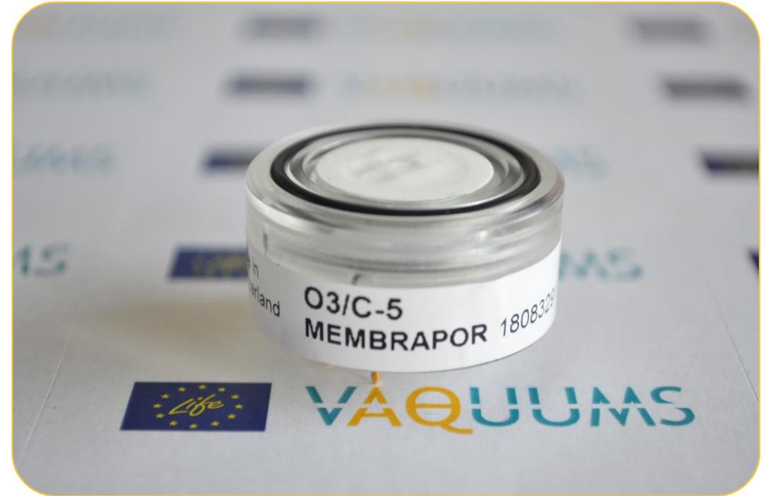
The Membrapor O3/C-5 is an electrochemical ozone sensor. It can measure concentrations between 0 and 5 ppm, with a resolution of 0.02 ppm. According to the manufacturer the compact series have the highest reliability and maximum performance in a compact housing. The sensor should be suitable for most applications.
