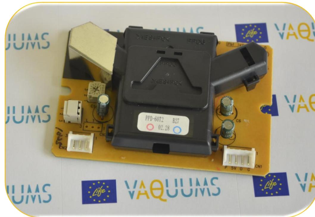
The Shinyei PPD60 detects air borne particles sized over 0.5  $\mu\text{m}$  based on the light scattering method. The air is self-aspirated by the air current generation mechanism with a built-in heater.
